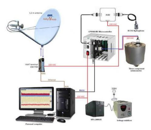
Fig. 2. Diagram of the station
